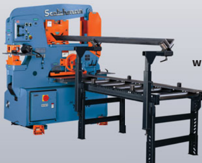
Multi-Loc Punch Gauging Extension: 36" & 85" (DD)
